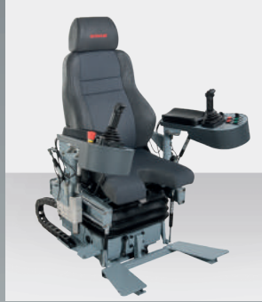
Crane control unit
